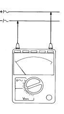
$^{\circ}$  Read off the measured value: in the case of DC voltage, on the two upper scales 0 ... 5 or 0 ... 15 V, A  $_{=}$  , in that of AC voltage, on the scales beneath 0 ... 5 or 0 ... 15 V, A  $\sim$  .
